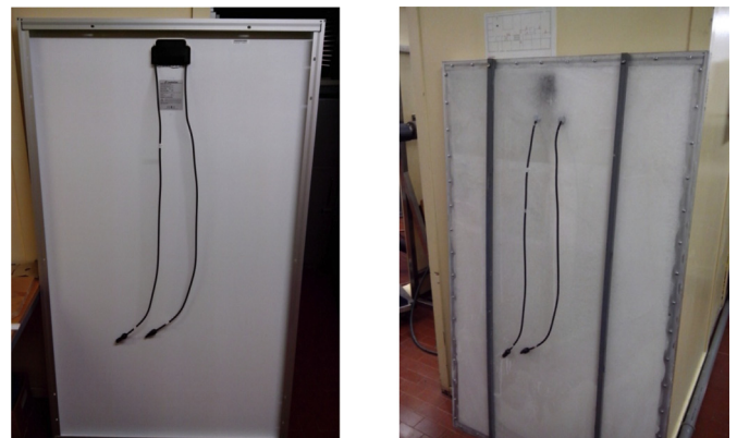
Fig. 1. Conventional PV panel before (left) modification and after (right) modification.
