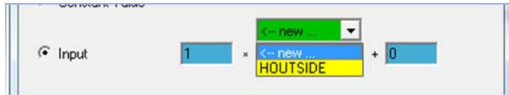
Figure 6: Creating a New Input for Ventilation
