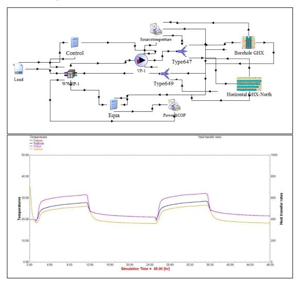
Horizontal Loop & Borehole in Parallel
