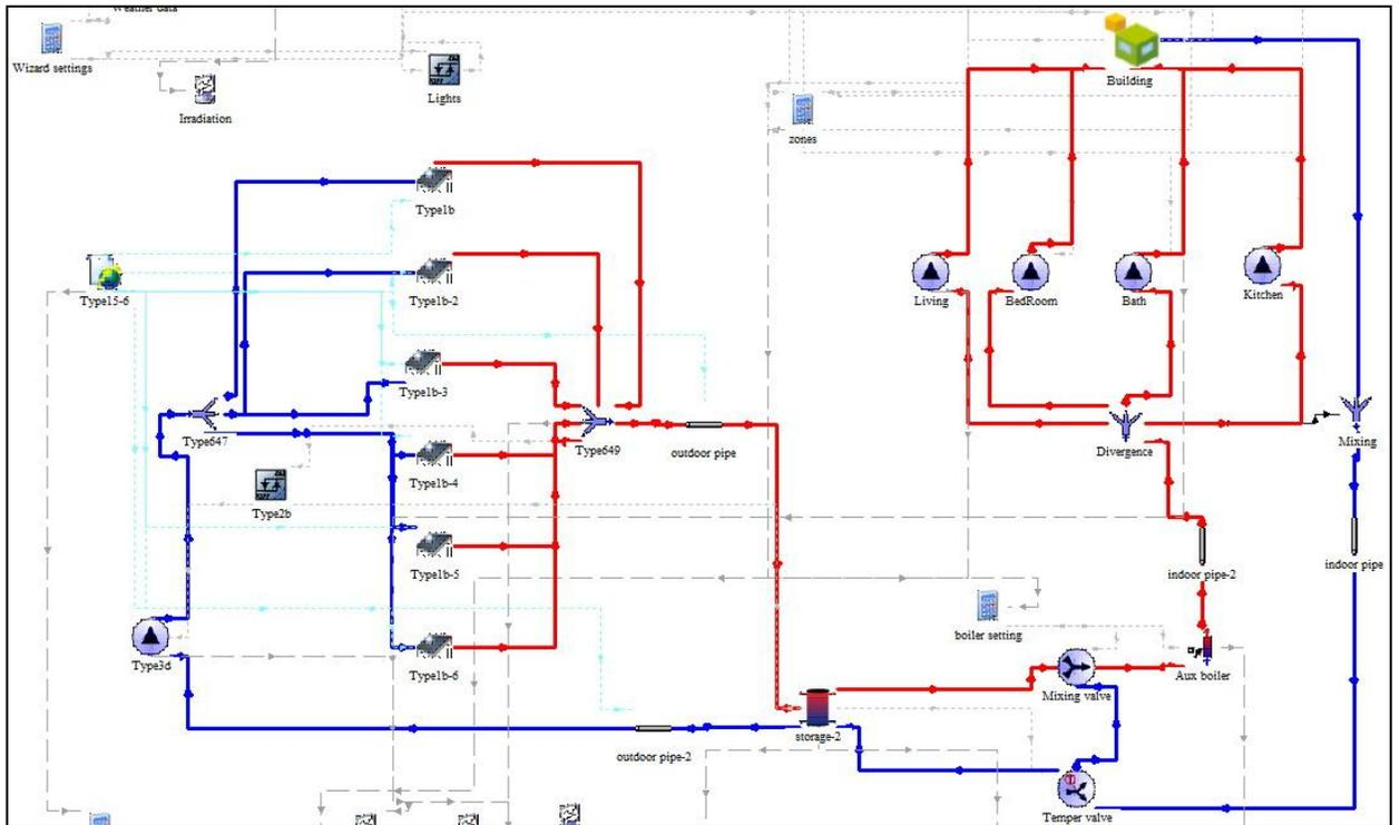
Figure 4: TRSNYS modelling of the solar system and the building
