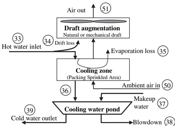
Fig. 3. GateCycle schematic of a cooling tower.
