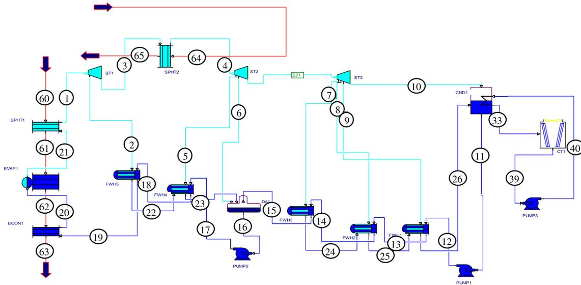
Fig. 1. GateCycle flow diagram 50 MWe Rankine cycle with wet heat rejection.
