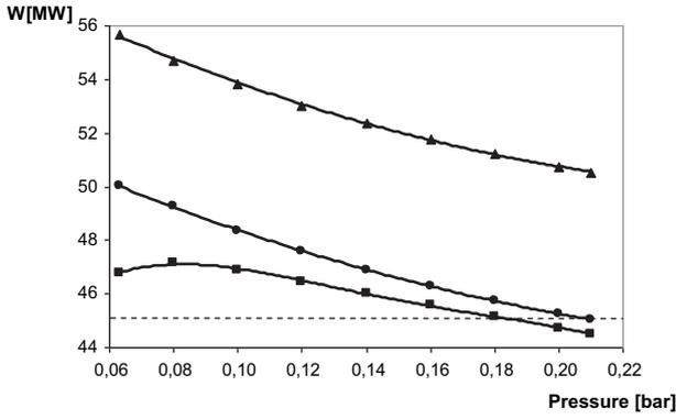
Fig. 2. Gross cycle power (▲), net cycle power with cooling tower (●) and net cycle power with air cooled condenser (■), versus condensing pressure (---- 45 MW).
