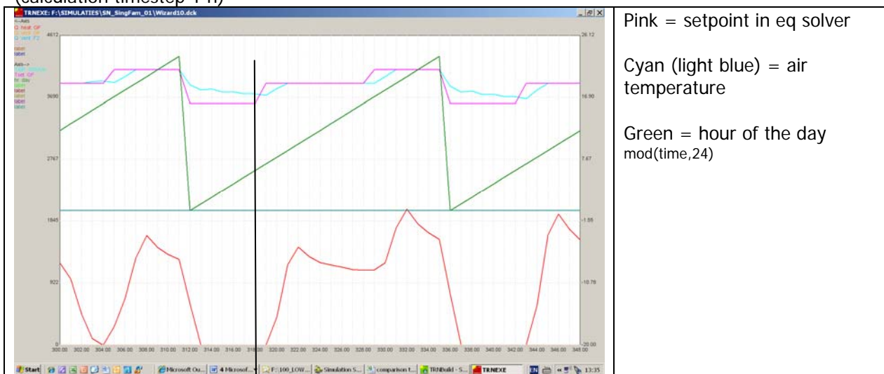
Figure 2: comparing the resulting indoor air temperature (pink) with the setpoint as produced with an equation solver.
