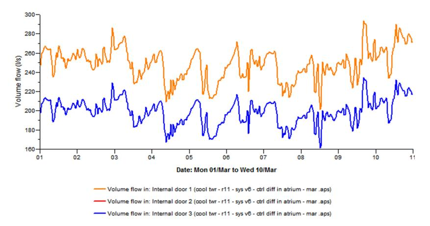
• Flow at two controlled discharge dampers in the UFAD supply plenum (controlled diffusers in MacroFlo are "doors" with formula profiles).
