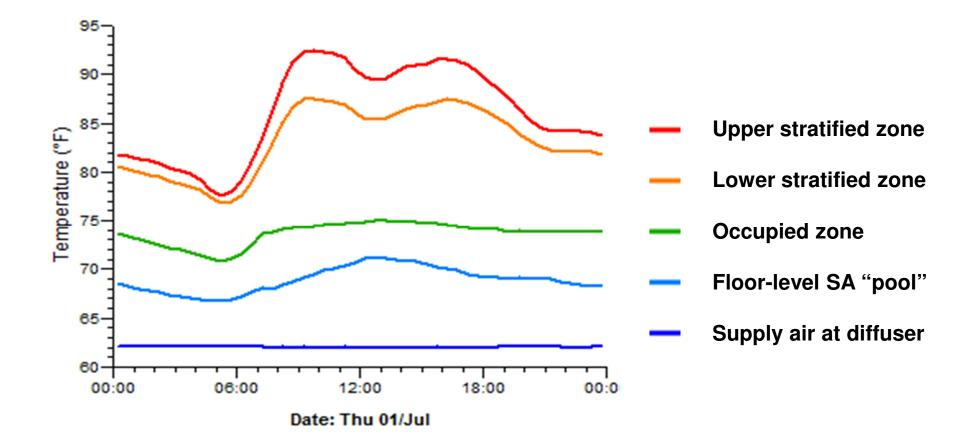
Zone temperatures for the zonal modeling method: 10-zone model with bulk-airflow network.
