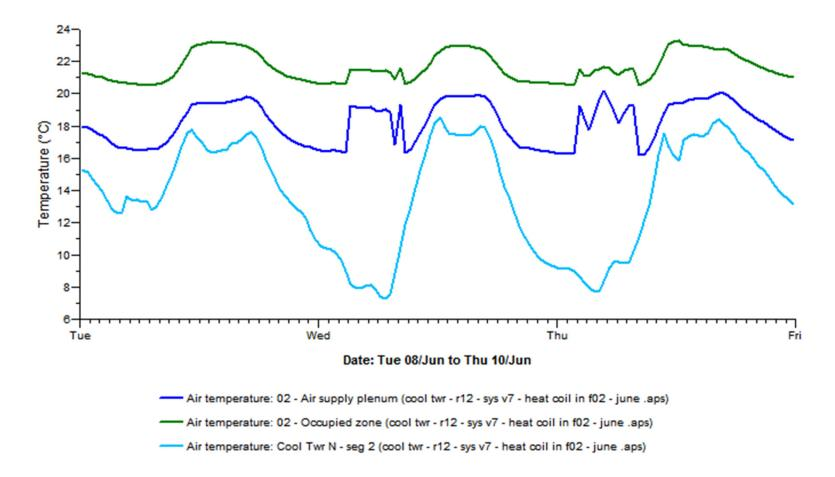
• Occupied zone temperature (green) is maintained by reducing flow from cool tower (light blue) to vent only and engaging floor plenum heating coil
