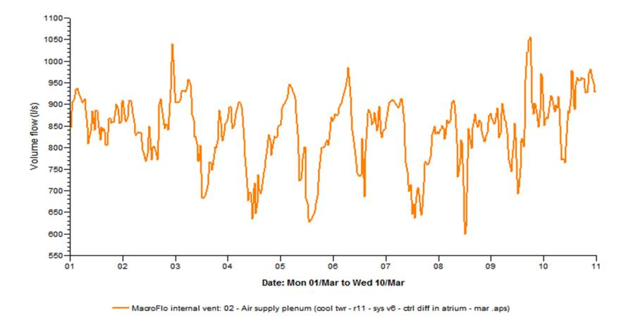
• Flow into the 2<sup>nd</sup>-floor UFAD plenum is controlled by dampers at the connection to the cool towers so that plenum can be heated in winter.
