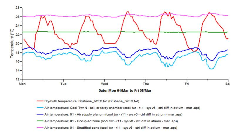
• Control of both coil LAT in towers and passive flow via dampers results in very tightly controlled space temperature and avoid excessive cooling.
