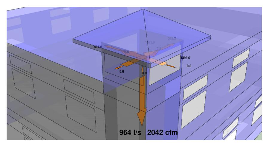
• Passive downdraft outflow from cooling coil cell of the tower (North and South towers shown) to the next cell or tower segment below.
