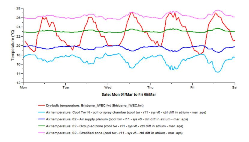
• Temperature in 2<sup>nd</sup>-floor occupied zone is slightly more variable as a result of heat transfer from RA below through floor deck into UFAD plenum.
