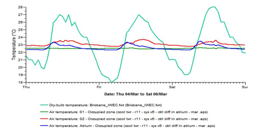
• Temperature in occupied zones (green, blue, and red lines) vs. outdoor temperature (light teal – Brisbane, AU, Mar 4-6).
