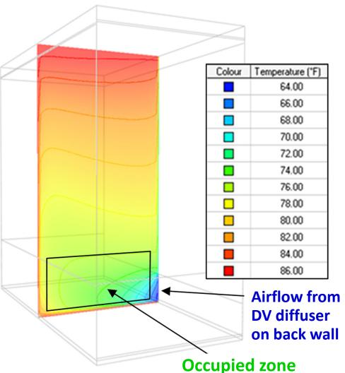
• Temperature at center of occupied zone was basis for comparison of airflow requirements at a given supply air temperature.
