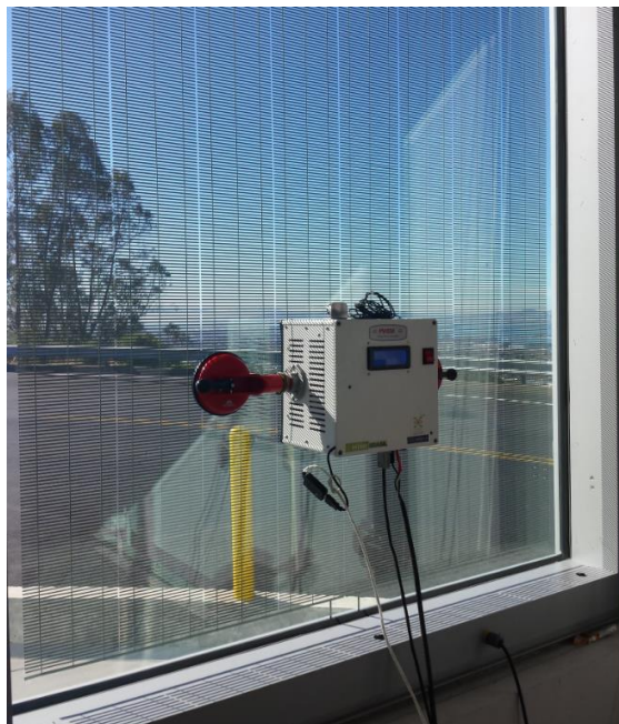
Figure 5 – PoWEM in action, measuring SHGC of a Commercial Window Glazing
