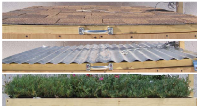
Figure 2: Four Roof Types: Asphalt Shingle, Corrugated Metal, Saturated Green (Vegetated) Roof and Dry Green (Vegetated) Roof
