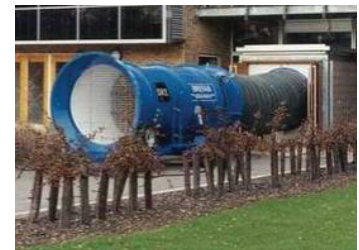
Figure F8. Trailer mounted door fan: 152,100 L/s (30,000 cfm) at 75 Pa.
