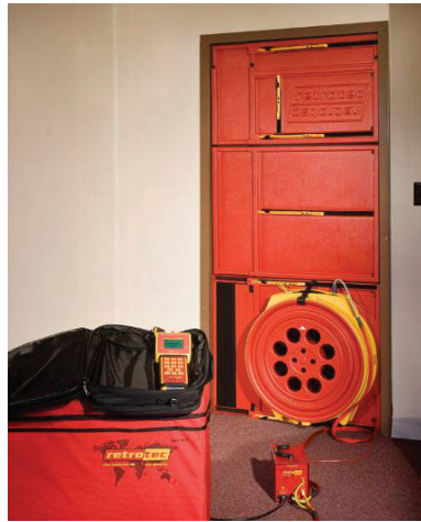
Figure F5. Commercial modular door fan: 121,700 L/s (24,000 cfm) at 75 Pa
