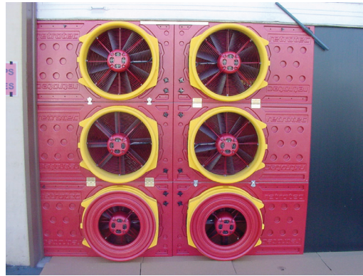
Figure F10. Portable commercial modular door fan: 243,360 L/s (48,000 cfm) at 75 Pa.
