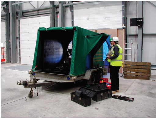
Figure F9. Trailer mounted high power fan: 253,500 L/s (50,000 cfm) at 75 Pa. Ideal for large warehouses.
