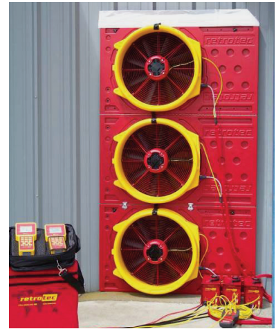
Figure F6. Large commercial modular door fan: 121,700 L/s (24,000 cfm) at 75 Pa
