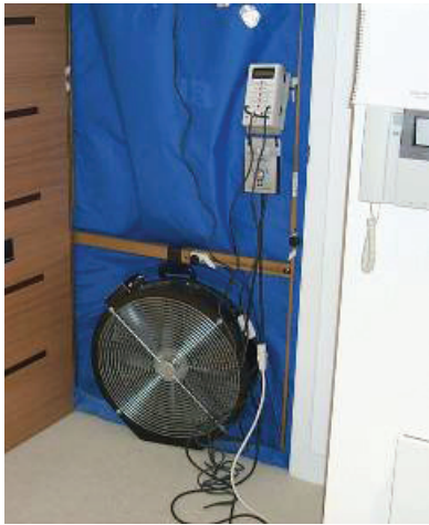
Figure F4. House testing door fan: 25,350 L/s (5,000 cfm) at 75 Pa
